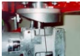
Elevator cam Picture # 34
