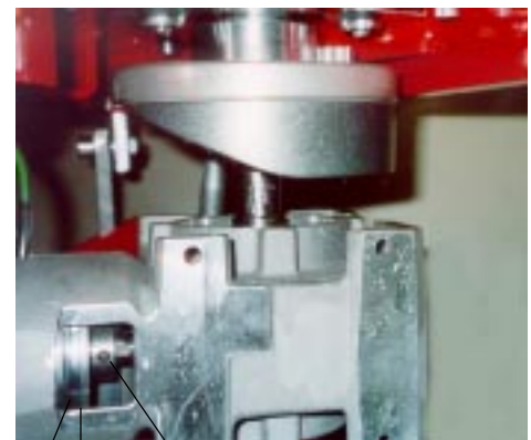
Stator Rotor. Adjustment gap
